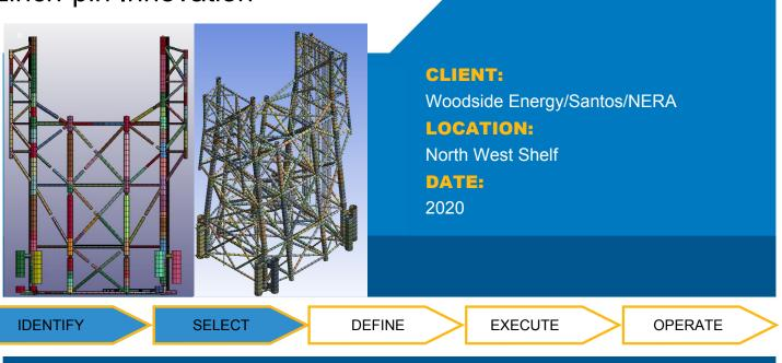
Linch-pin, with support from Santos and in collaboration with Woodside Energy and the National Energy Resource Australia organisation (NERA), has developed a world first concept for collapsing a Jacket in-situ - flat onto the seabed.
