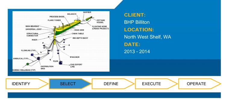
The Griffin Field is sited in 130m of water located on the North West Shelf, South-West of Barrow Island. The Griffin Field facilities include the RTM type of Single Point Mooring (SPM) terminal, subsea flowlines (production, gas lift and control umbilicals), subsea distribution skids and wells. An 8" Gas Export Pipeline (GEP) had also been installed to transport gas from the field to an onshore gas plant.
