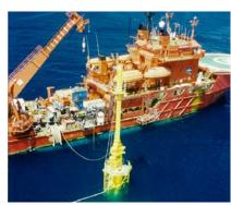
Lending itself to installation and removal of items such as Mid Depth Buoys etc, Linch-pin's innovative chain puller allows full control of the buoyant structures to be installed or removed, thereby reducing the HSE risks associated with the operations.
